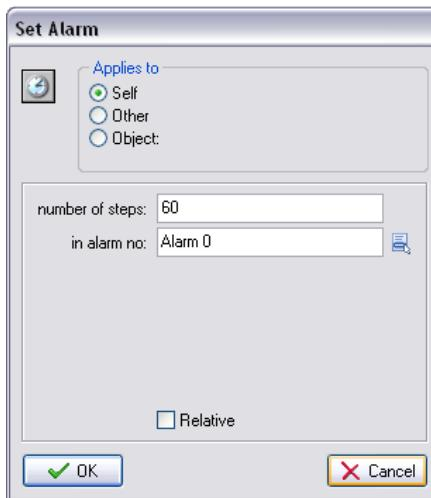
This will set Alarm0 to go off in 60 steps (~ 2 seconds at standard game speed). In this case, **Relative** can be used to add time to an alarm that is already set. The Alarm system in Game Maker works a lot like the timer that we used to kill the player if they don't get to the exit in time in Temple of Locks.
